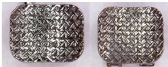
Fig 5. Stainless steel : before and after sandblasting
