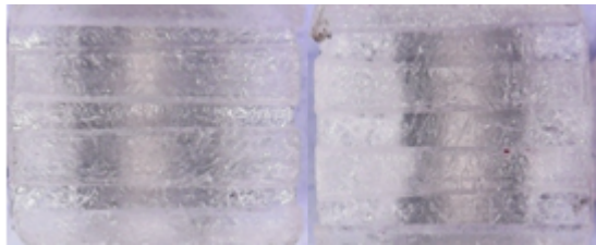
Fig.3. Composite material : before and after sandblasting
