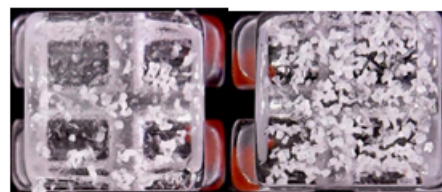
Fig 2. Monocrystalline alumina: before and after sandblasting (a better retention surface was obtained)
